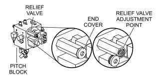
Figure 53. Pitch Pressure Adjustment
